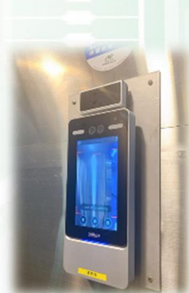
Caption: Access Controller with temperature measurement 圖片說明：探熱測溫門禁系統
